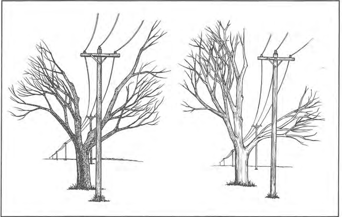
Figure 10. Directional pruning causes trees to assume different shapes depending on the location of utility facilities.
