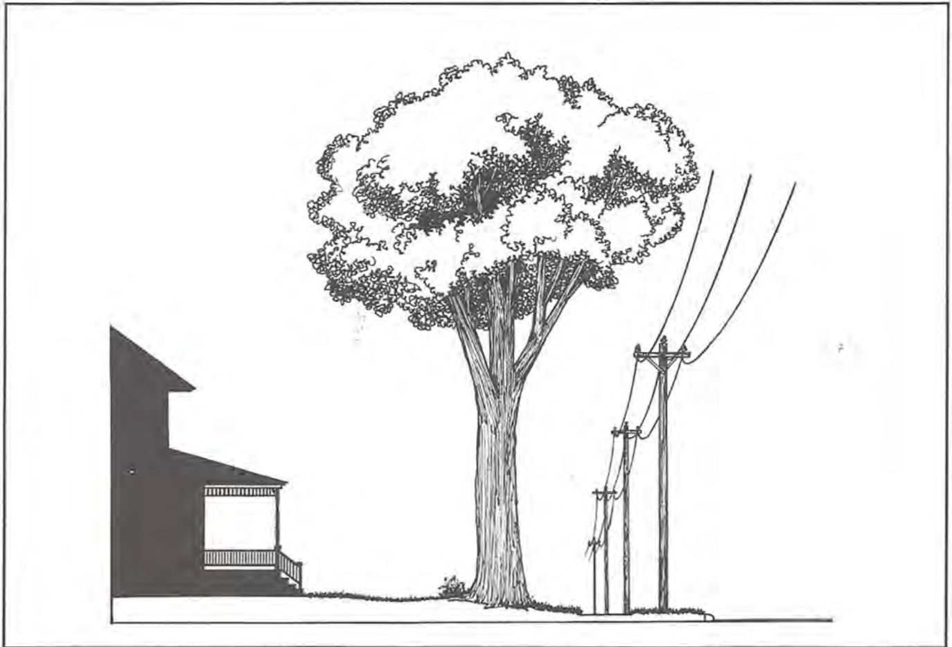
Figure 11. Removal of overhang may or may not be necessary depending on the type of utility facility, tree species, or other factors. Overhang is never acceptable over high-priority facilities such as high-voltage electric transmission lines.
